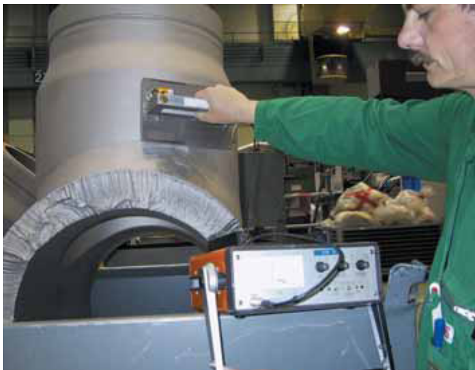
Figure 11. Measurements with surface contamination monitors on metallic components (EON, 2008).
