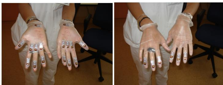
Fig. 3. The operator's gloves equipped with doseimeters for the dosimetric study in WP4.
