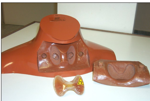
Figure 1. IRSN thyroid phantom for intercomparison (left), SCK-CEN thyroid phantom for calibration (right).
