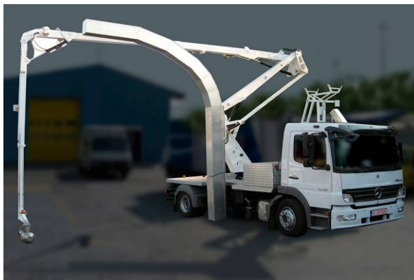
Fig. 3. View from the right of the ROBOSCAN 1M in scanning position.
