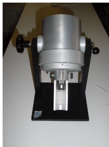
Fig. 6. Lead shielding for F-18.
