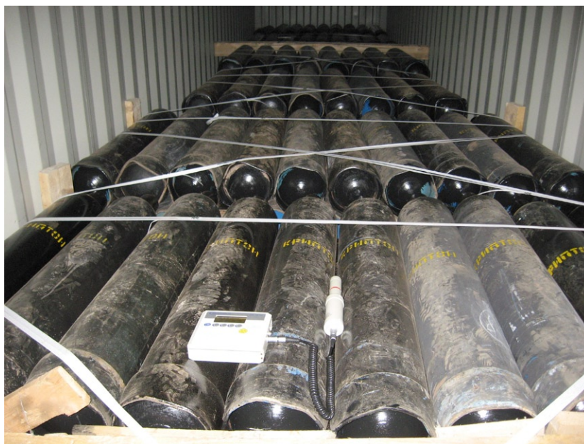
Fig. 1. Cargo of steel cylinders containing pressurized krypton gas, with the dose rate meter in measurement position.
