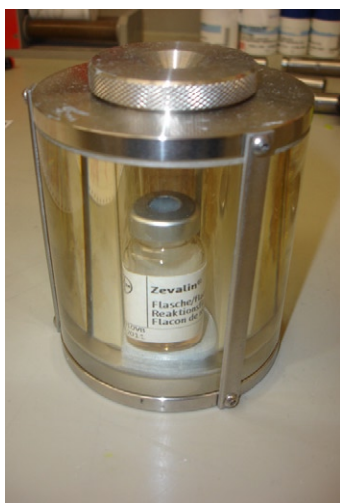
Fig. 4. Vial Plexiglas shielding for beta emitters.
