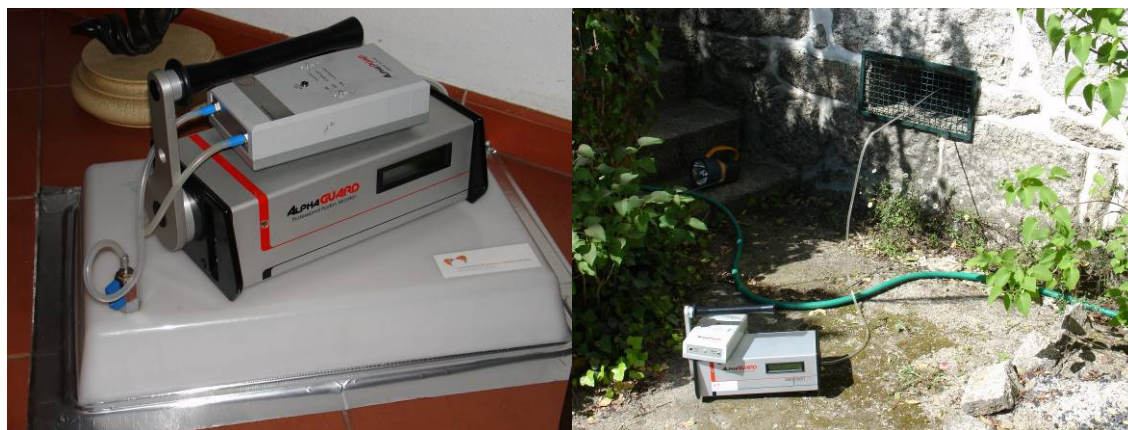
Fig. 2. Radon-box technique measurement with Genitron-Saphymo™ AlphaGuard Pro (left) and radon concentration measurement in a crawl space (right).
