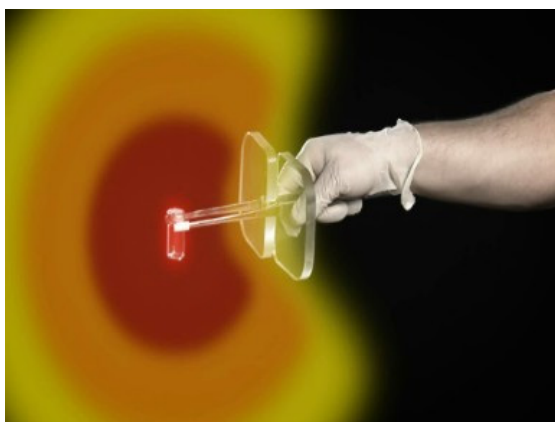
Fig. 7. Tweezers with Plexiglas beta shielding.
