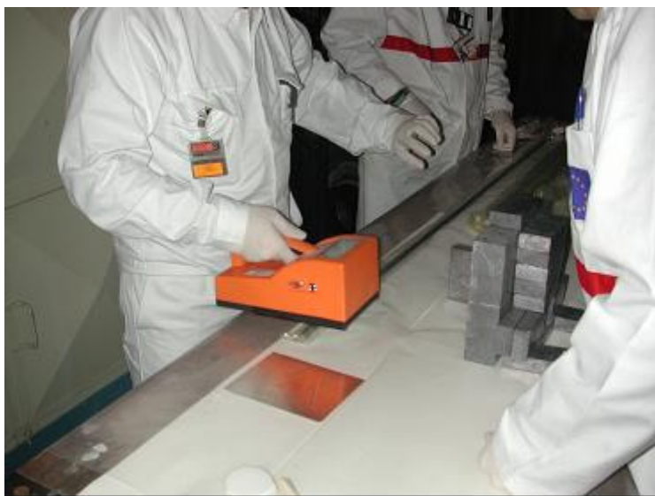
Fig. 1. Radiological control of surface contamination with a Berthold LB124.
