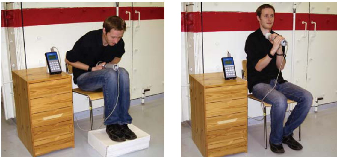
Figure 4. Left: "Lap geometry" for whole body measurement with portable gamma spectrometer. Right: Measurement of ^{131}\text{I} in the thyroid. These photographs illustrate the method, but when responding to an incident, additional measures would need to be employed, i.e. the detector would be wrapped in plastic film, and the subject would wear disposable gloves. Photos: STUK.
