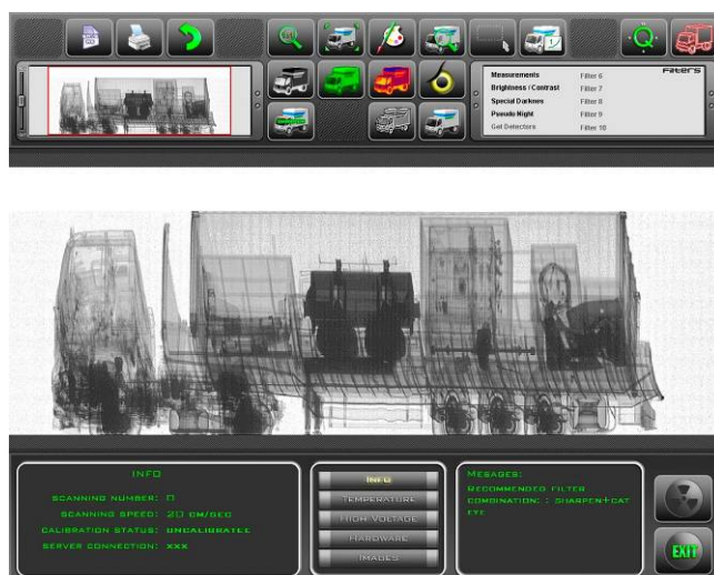
Fig. 5. View of radiography of the scanned truck in imaging software application.
