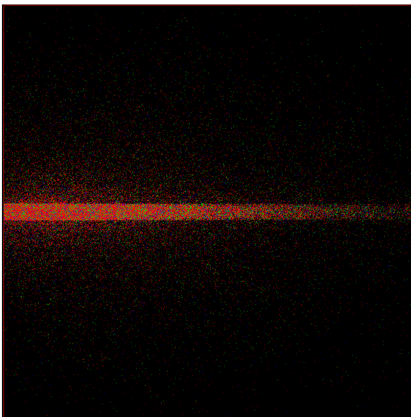
Fig. 7. Simulation of 100 000 photons emitted from a 4 mm (diameter) disk according to the energy distribution measured for I-125 brachytherapy seeds. The simulated volume consists of 10 \times 10 \times 10 \text{ cm}^3 of water vapour at a density of 0.7320 \text{ g/cm}^3 . Different types of interactions are colour-coded as follows: red, photoelectric effect; green, Compton scattering; blue, Rayleigh scattering.
