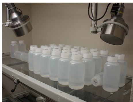
Fig. 1. The KIT whole body counter. A bottle phantom representing a 70kg person is placed on the bed. Only the upper two detectors can be seen in this figure.
