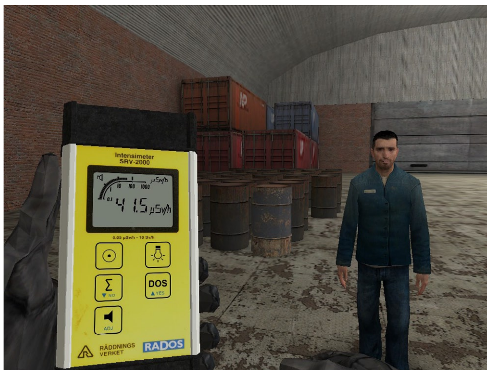
Fig. 1. A screenshot from RadiaX. The SRV-2000 is virtually held in the trainee's left hand and the buttons are selected using specified keys or mouse buttons. Each button is highlighted for a second when selected.
