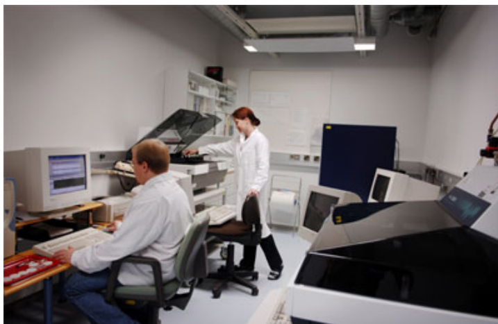
Fig. 3. Activity concentrations of tritium, Rn-222, C-14 and Sr-90 are determined using Guardian 1414 liquid scintillation spectrometer.
