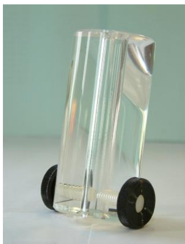
Fig. 5. Syringe shielding for beta emitters.
