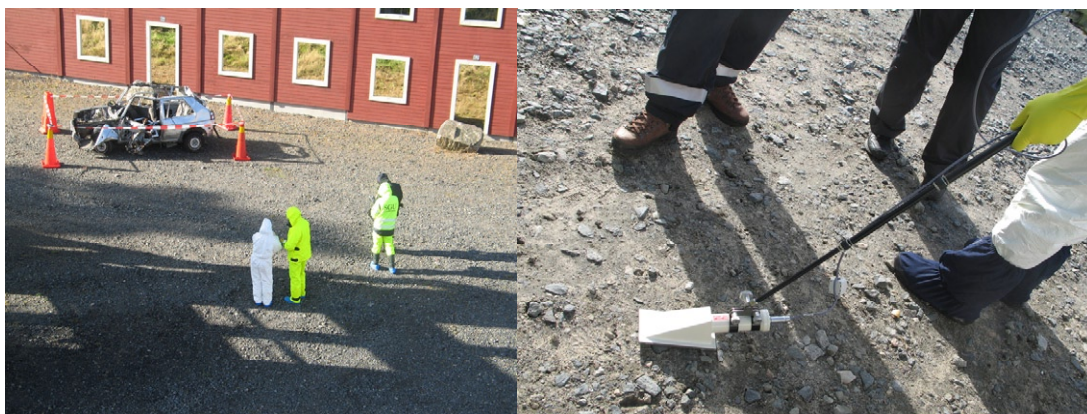
Fig. 3. Left picture showing a team assessing the radiation field with the supervisor being the person i yellow to the left. Right picture showing the optimal geometry in search of ground contamination and hot particles.
