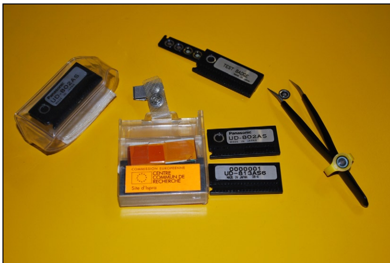
Fig. 1. Personal dosimeters at the JRC: wrist, whole body and ring.
