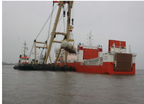
Fig. 2. Steam generator during loading on a ship.
