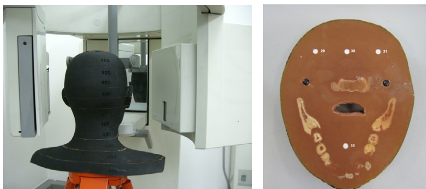
Fig. 1. Alderson-Rando phantom positioned inside the panoramic unit (left) and slice 7 with four TLD positions 29 to 32 (right).
