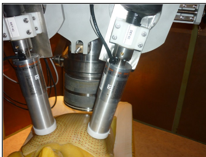
Fig. 1. The geometry of the WBC measurements on GE Healthcare staff.
