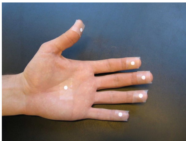
Fig. 9. TLD for the determination of the maximum dose to extremities.
