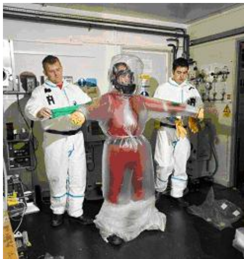
Fig. 16. The new pressurised suit with integrated air fed respirator.
