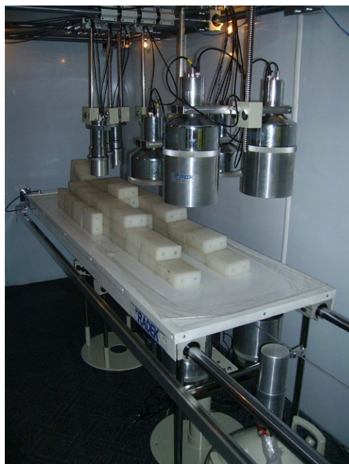
Fig. 5. Detectors view inside the chamber with couch and with phantom.
