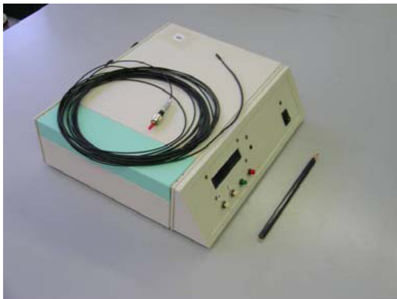
Fig. 1. Picture of a prototype of the acquisition unit (ELSE S.r.l., Italy) with the RL fibre.
