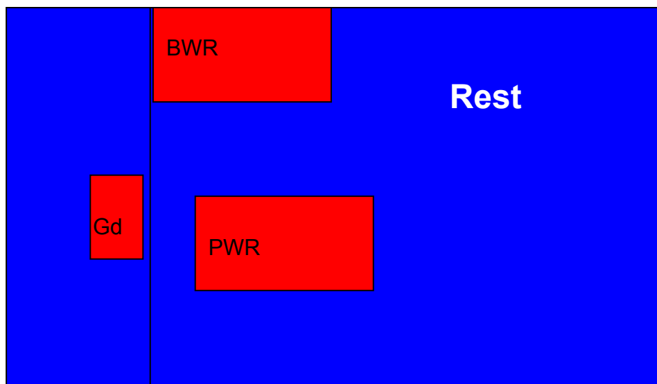
Fig 3. Example of survey plan on the roof. Areas around the stacks are red (class 1). The rest of areas are class 2 because they are near areas class 1.
