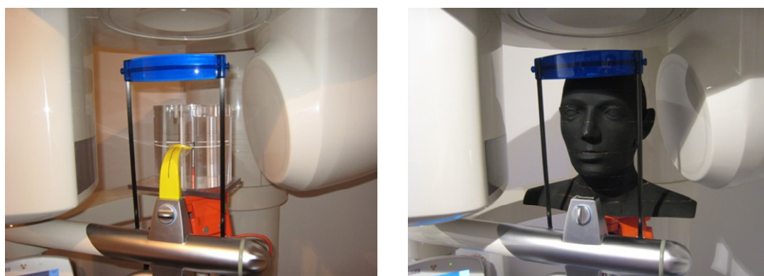
Fig. 2. Phantoms positioned inside the DVT, cylindrical PMMA phantom (left) and Alderson-Rando head phantom (right).
