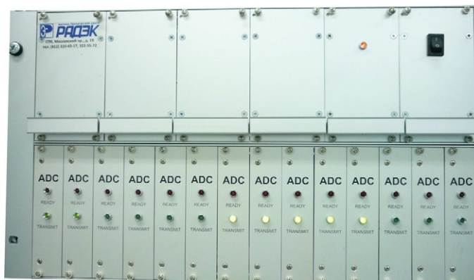
Fig. 6. View of 14 analyzers MD-198 from the front side in the control cabinet.
