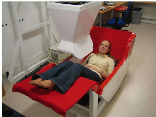
Figure 2. The present measurement set-up in the mobile unit. The modified chair is made of lead. The white shadow shield is also made of lead from “waist” down. Upper part is made of steel covering the detectors and supporting them.
