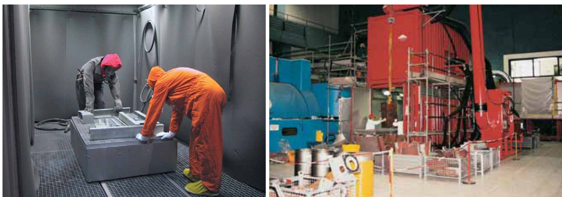
Figure 9. Left: loading of material into the grit blasting caisson. Right: the grit blasting container from the outside (E.ON, 2008).
