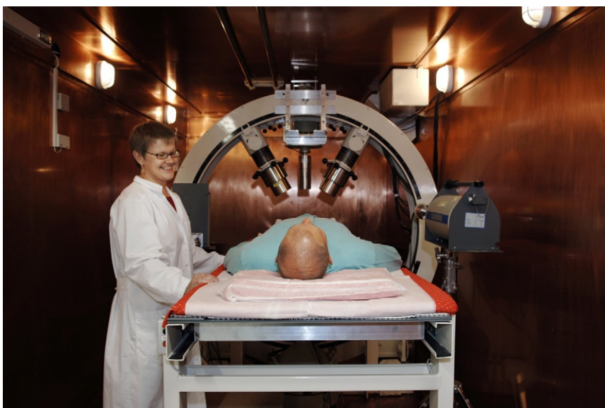
Figure 3. Inner view of the Ironroom. The indoor whole body counter uses HPGe and NaI detectors, some of which are visible above the person being measured.
