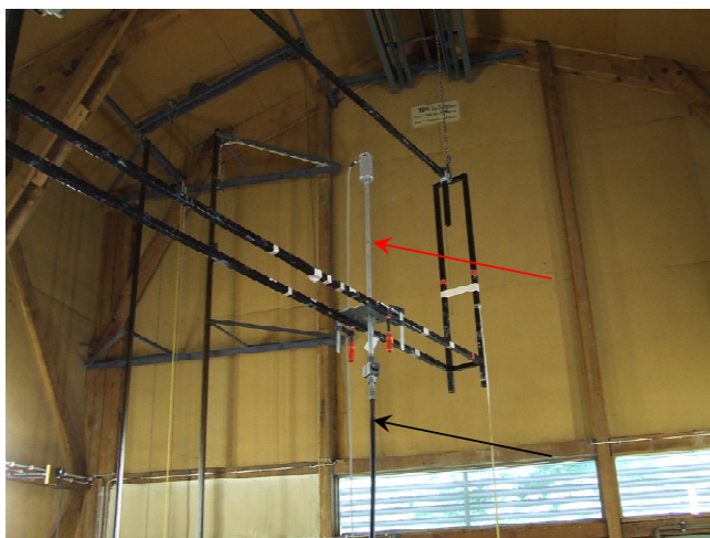
Figure 3. The irradiation device in the wooden irradiation hall: The red arrow indicates the position of the moved out Cf-252 source in a thin aluminium cylinder. The source can be moved to this place in a flexible tube from a shielded storage place (black arrow). The black frame of a provisional hoist system and parts of the wooden hall are visible too.
