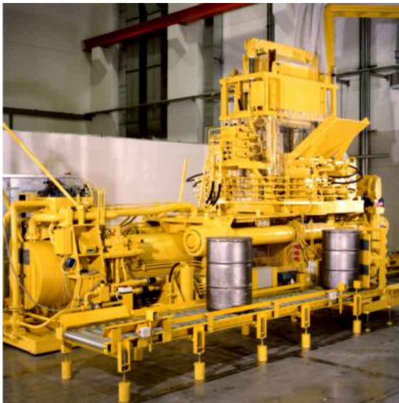
Figure 10. Volume reduction of 200 l drums (FAKIR supercompaction facility, GNS).
