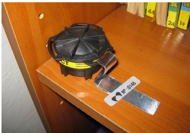
Fig. 1. CR39 passive detector secured with a VOID label.
