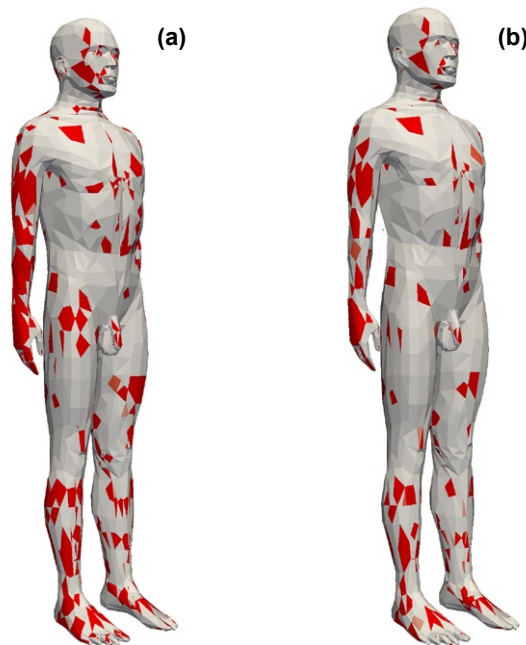
Fig. 8. Bad elements selected by “a priori” criteria : geometrical (a), spectral (b) for the A-Phi formulation.
