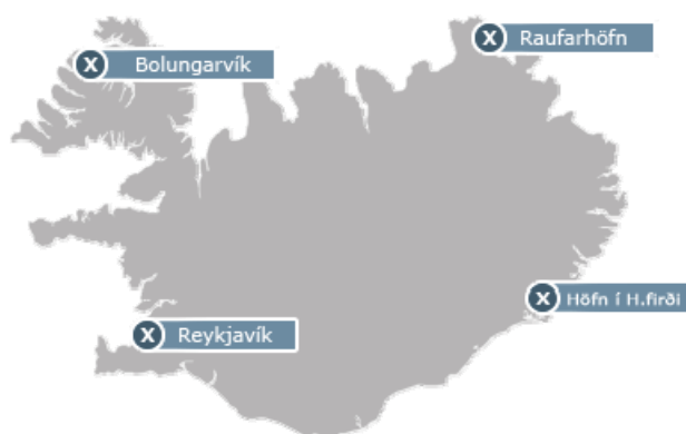
Fig. 1. Locations of IRSA's four gamma monitoring stations. Gamma background, rainfall, temperature, pressure, windspeed and wind direction is collected at these sites.
