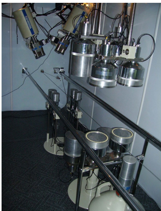
Fig. 4. Detectors view inside the chamber without couch.
