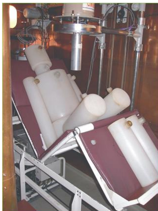
Fig. 1. Whole Body Counter in LPD with BOMAB phantom during calibration.
