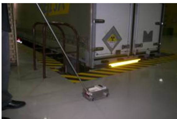
Fig 3. Device used to scan surfaces in order to find contamination spots.
