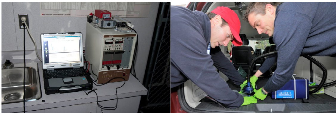
Figure 1. DAAFS spectral acquisition equipment (left) and sampling of clothing from pre-Olympic Exercise with Lilliput vacuum and nozzle (right).
