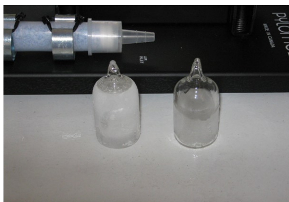
Fig.2. Flame sealed ampoules: left – LS; right - gas.
