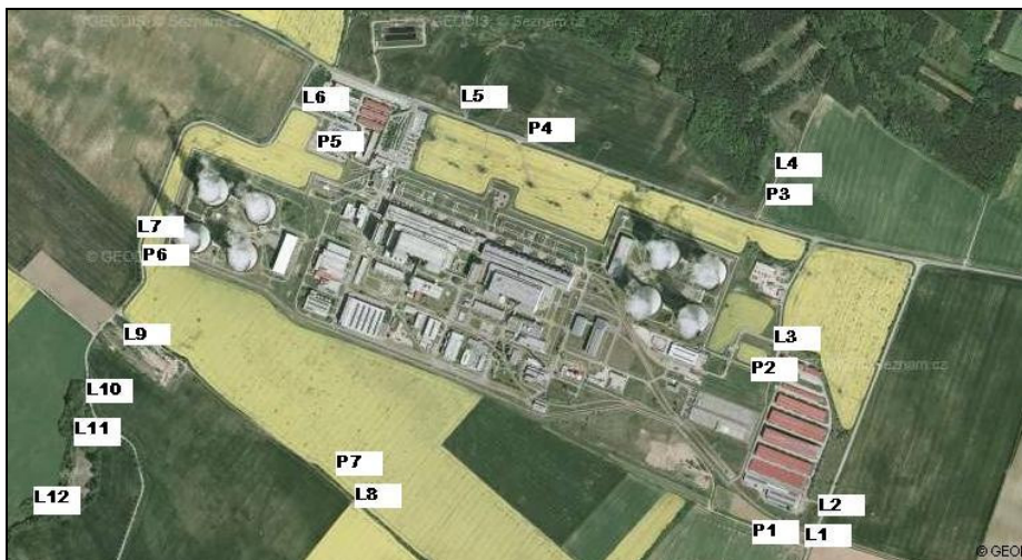
Fig. 1. Nearest sampling points around NPP Dukovany for HTO activity monitoring in air moisture. P – prompt sampling, L – long term period of sample cumulation.
