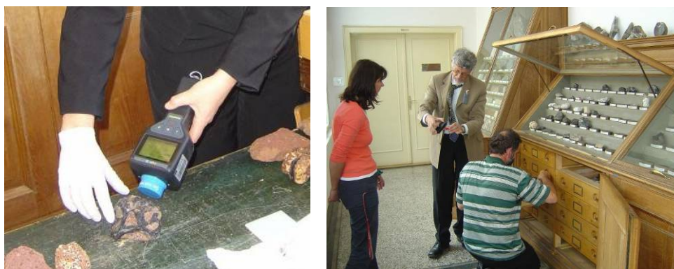
Fig. 2. Measurements of the photon dose rate of the geological specimen using Fielddos and a use of a radiation pager for identification of elevated dose rates in 2007.
