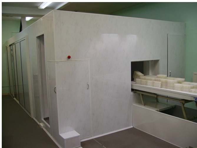
Fig. 3. Chamber of spectrometer of human radiation inside view.
