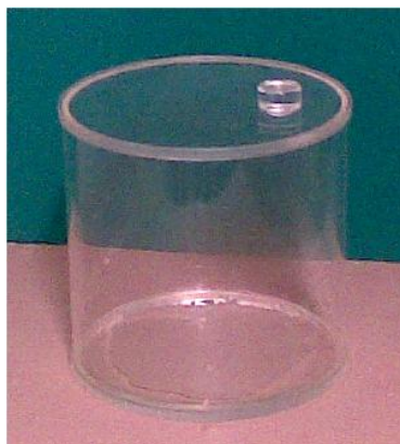
Fig. 2. The cylindrical calibration phantom for eye-lens operational quantity dosimeter testing.
