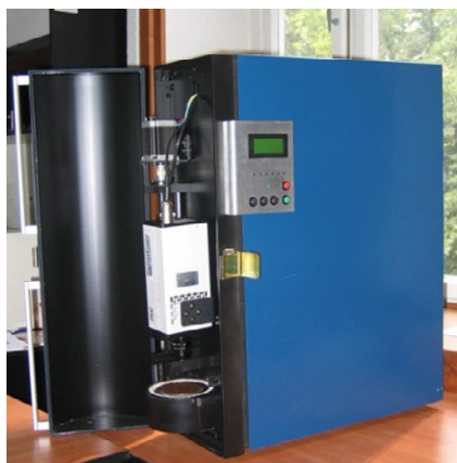
Fig. 2. TLD reader with CCD camera developed in Insitute of Nuclear Physics PAN.
