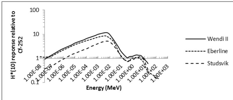
Figure 2:  $H^*(10)$  response relative to Cf-252 of the ambient monitors used in the measurement campaign.
