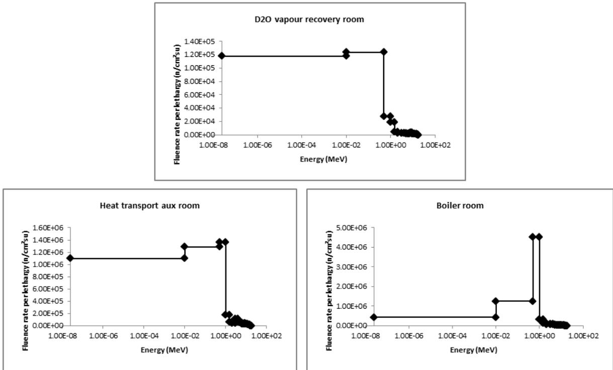
Figure 3: The spectra obtained with the Nprobe are in general soft spectra. An exception to this is the spectrum obtained in the boiler room, where there is a rather large contribution from neutrons having energy from 0.5 to 1 MeV.
