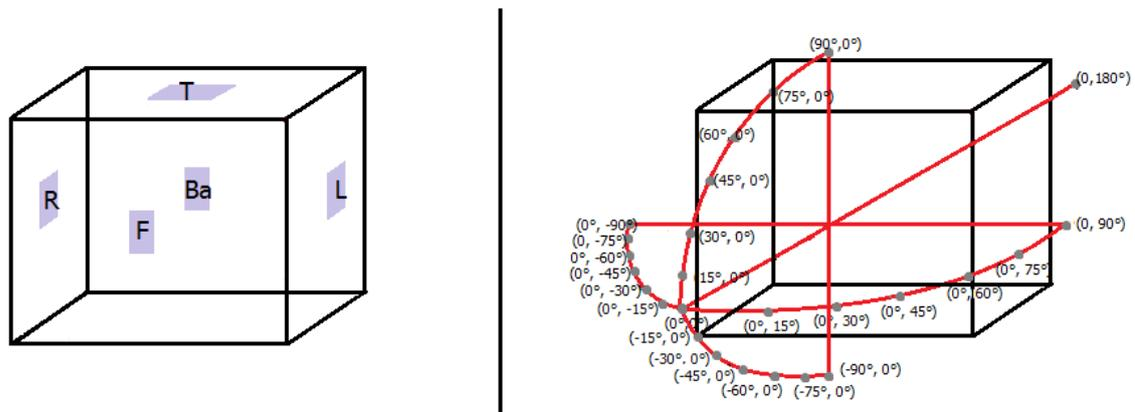
Figure 1: Both active and passive dosimeters were placed on all sides of a slab phantom (left figure) to estimate the angular distribution of the neutron fluence incident in different directions  $P(\vartheta, \phi)$  (right figure). This latter was done using linear interpolation techniques under the assumption that the energy distribution remains the same in all orientations.
