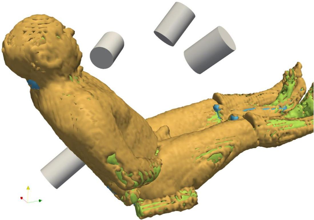
Figure 5 – Position of the detectors in the final WBC configuration.
