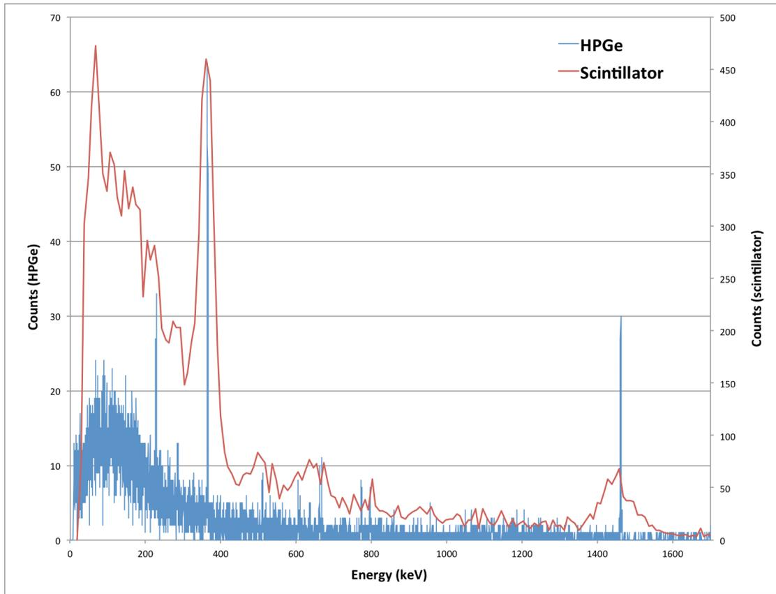
Figure 7 – Comparison of scintillator and HPGe detector spectra (not to scale).
