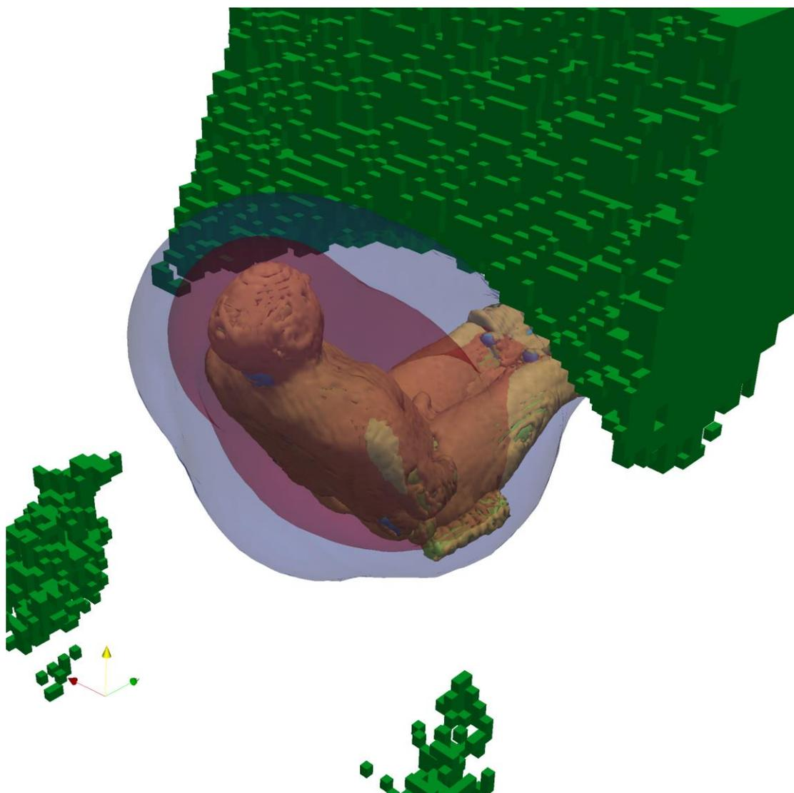
Figure 2 – Plot of the three phantoms used (overlapping each other) and of the iso-flux surfaces resulting from  $^{40}\text{K}$  sources distributed in several organs of the phantoms. The green region represents the volume of space where the standard deviation among the detection efficiencies for  $^{40}\text{K}$  in the different organs is lower than 20%.
