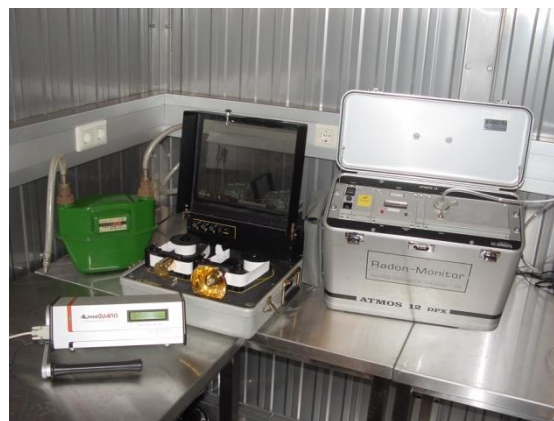
Fig. 8: Radon monitors in the BEV radon chamber
