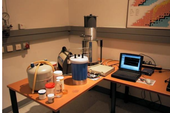
Fig. 7. Metrological control of a gamma-ray spectrometer
