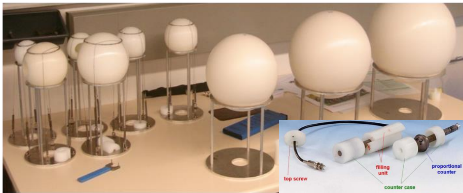
Figure 5. The CIEMAT BSS: bare, 3", 3.5", 4", 4.5", 5", 6", 7", 8", 9", 9.5", 10" and 12". Polyethylene density, determined by PTB: average 0.955 \text{ g}\cdot\text{cm}^{-3} .
