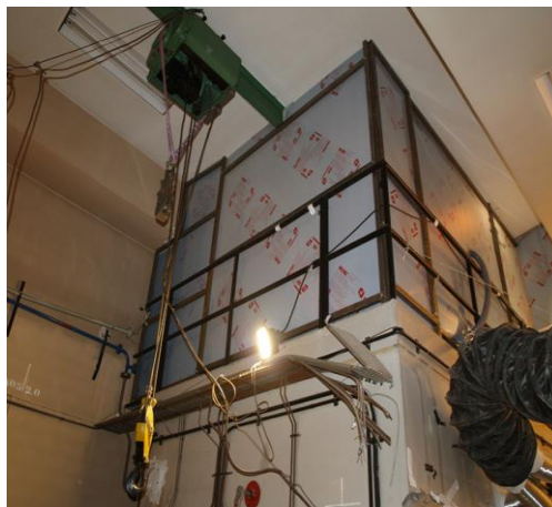
Rigid confined enclosure (CIEMAT)
