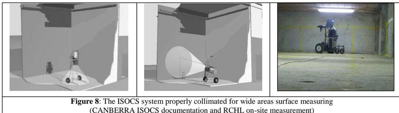
**Figure 8:** The ISOCS system properly collimated for wide areas surface measuring (CANBERRA ISOCS documentation and RCHL on-site measurement)
