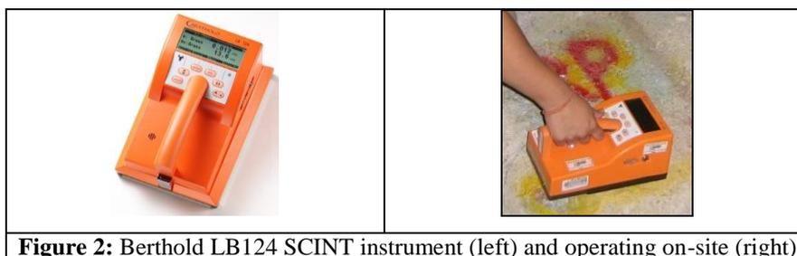
**Figure 2:** Berthold LB124 SCINT instrument (left) and operating on-site (right)
