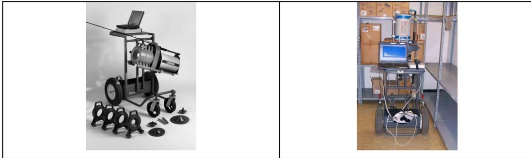
**Figure 3:** The ISOCS system with all its available components (left) and operating on-site (right)
