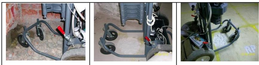
**Figure 7:** Near surface measurement with in situ gamma spectrometry
